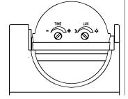
Turn LUX knob to minimum anti-clockwise, if you test it when the ambient light is more than 3LUX, the induction load would not work after the load stops working; the load should work if you cover the detection window with opaque object (towel etc), it would be regular the load stops to work within 7-13sec under no induction signal condition.
